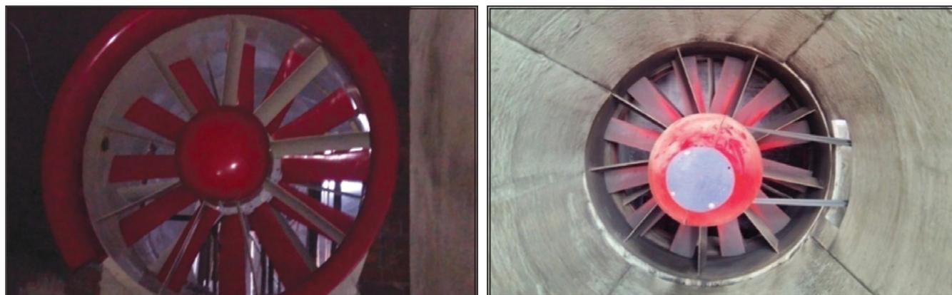
Large Diameter Ventilation Fan (1.8 m dia) installed at Gumgaon Mine
