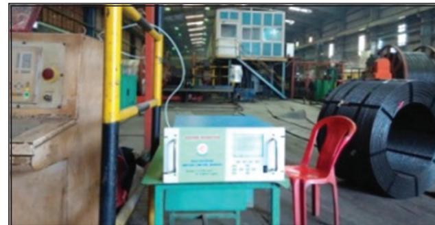
Indigenous portable Ozone Monitoring System for measurement of Real Time Ozone Concentration in and around Industrial area of Ranchi.
