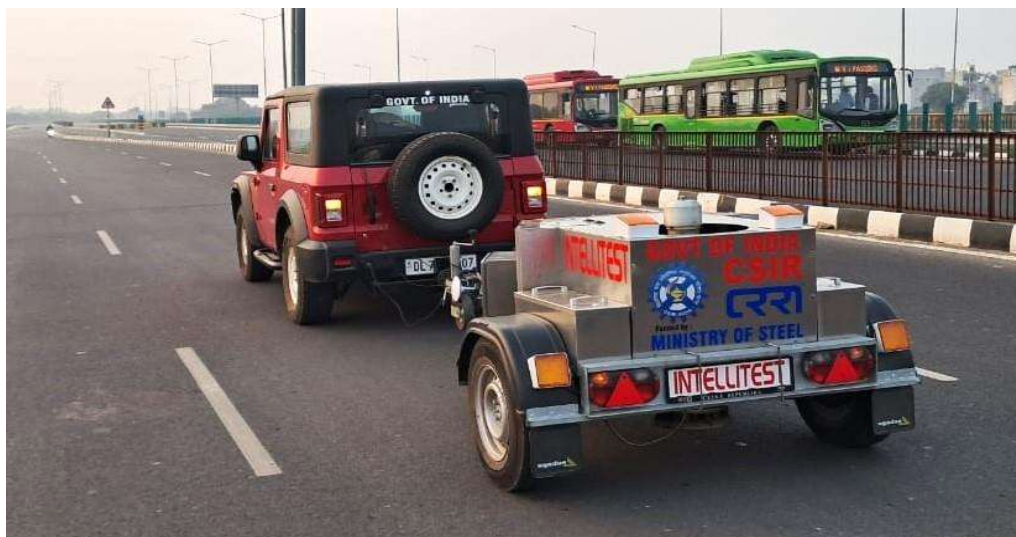
Photo A.10: Structural evaluation using Heavy Weight Deflectometer
