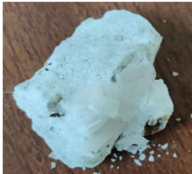
Photo 3.10: Tufa formation on BOF steel slag aggregate surface
