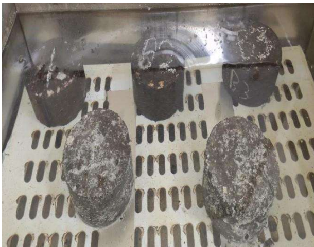
Photo 3.3: Cracked Bituminous mix, Marshall Test specimens at 60° C temperature in water bath due to volumetric expansion of steel slag
