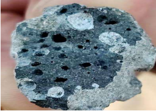
Photo 3.1: Lime Pocket in Steel Slag
