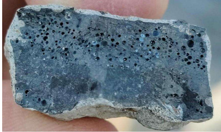
Photo 3.6: Porous Structure in steel slag at Macroscopic level
