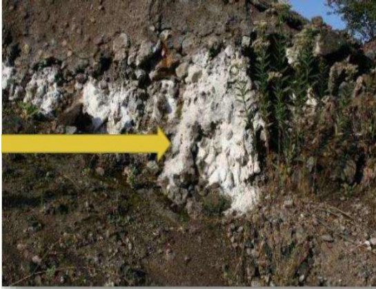
Photo 3.7: High pH leachate from slag dump
