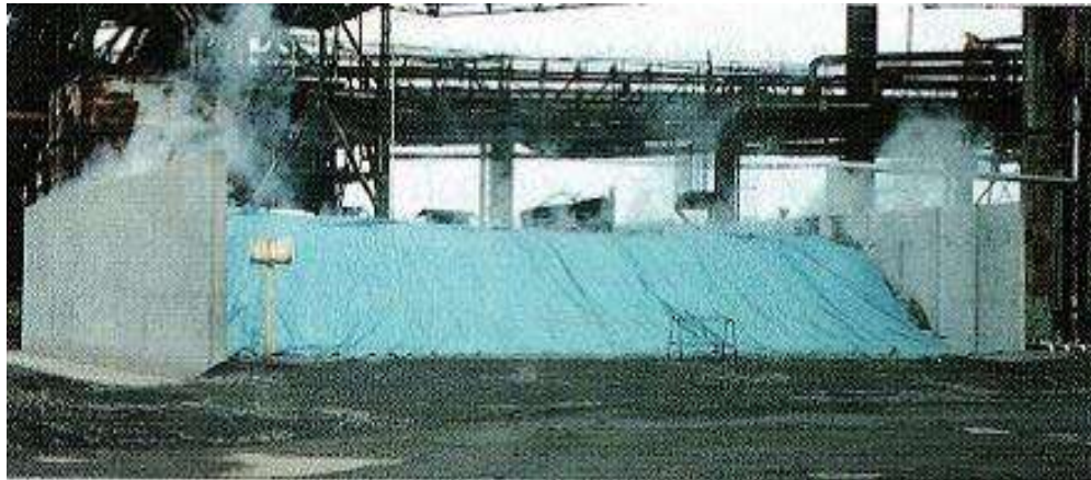
Photo 4.2: Large scale steam aging facility (Nippon Steel & Sumitomo Metal Technical Report No. 109 July 2015)
