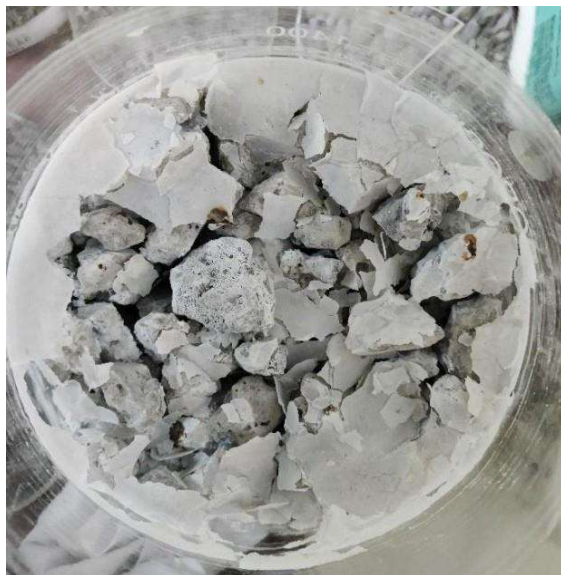
Photo 3.10: Tufa formation on BOF steel slag aggregate surface
